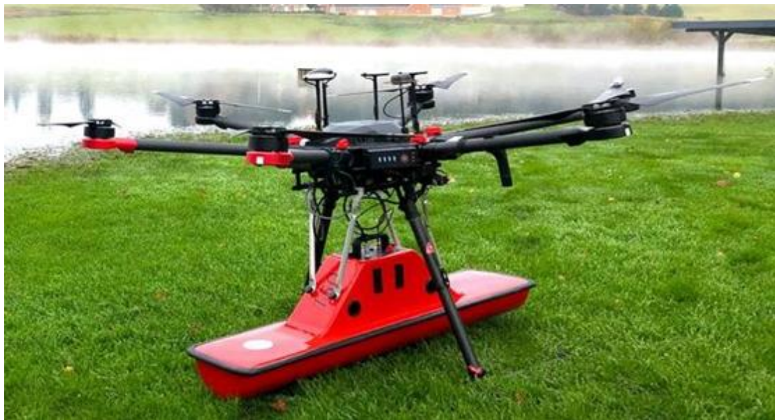
Fig. 2 Drone based ground penetrating radar GPR.
