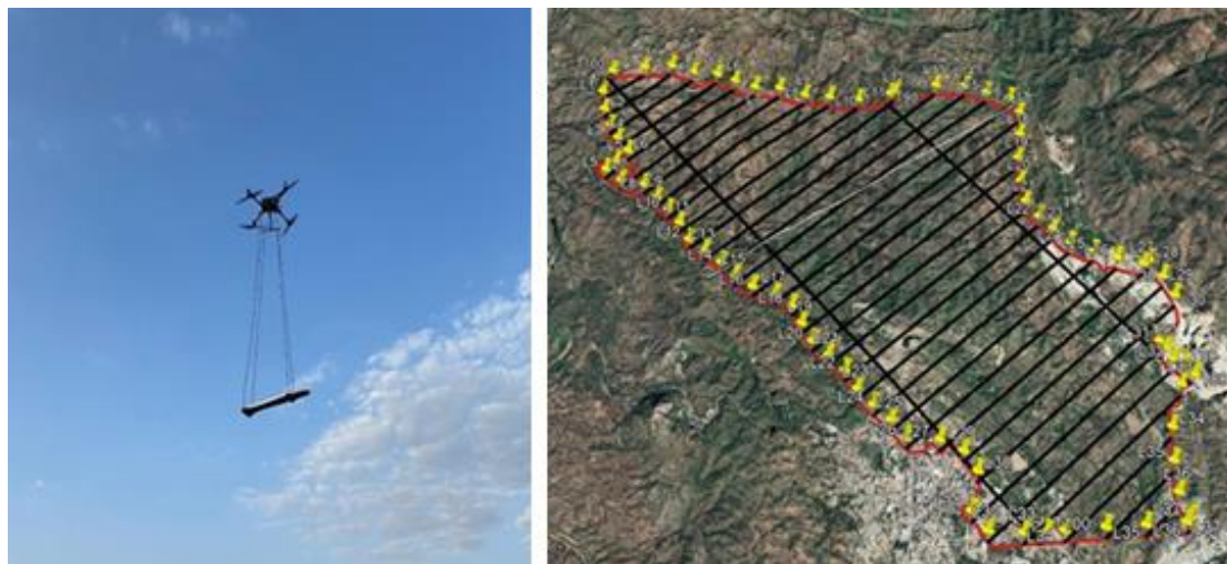
Fig. 1 (Left) Drone Based Magnetometer MagArrow. (Right) Illustration of flight path.
